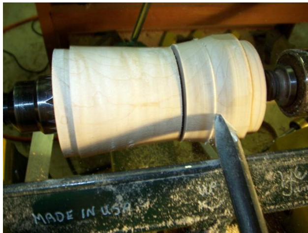
Shaping the Box Before Completing the Parting Cut
