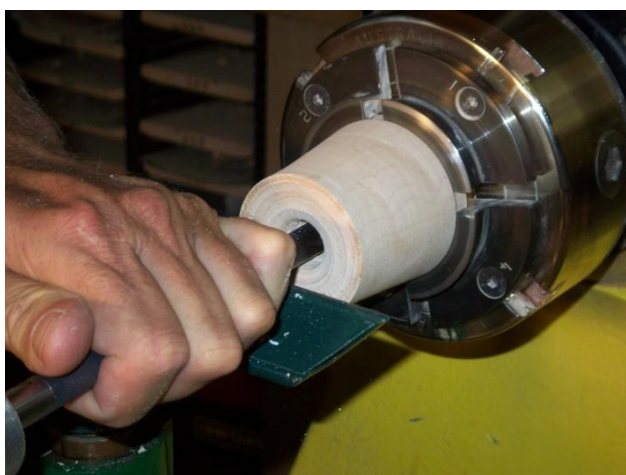
Drilling the Base
