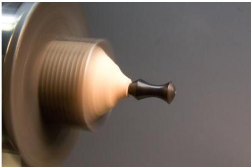
Regardless of how you get there, the mandrel should securely hold the finial to be finish cut, sanded, and finished appropriately. Care in creating the mandrel, including a shoulder to seat on for accuracy, allows the work run true.
