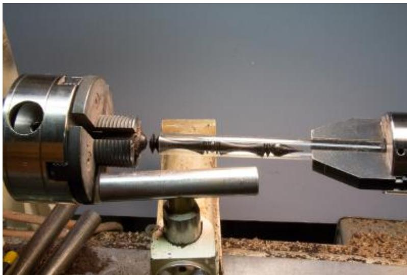
This is a pretty simple yet very powerful concept. A simple plastic tube, cup or any vessel that can be held, placed so it surrounds the work as it is parted off frees your hands and your mind. Using this and the toothpick (or anything else) in a drill chuck to catch any piece with a hole when parting off has many applications in turning.
