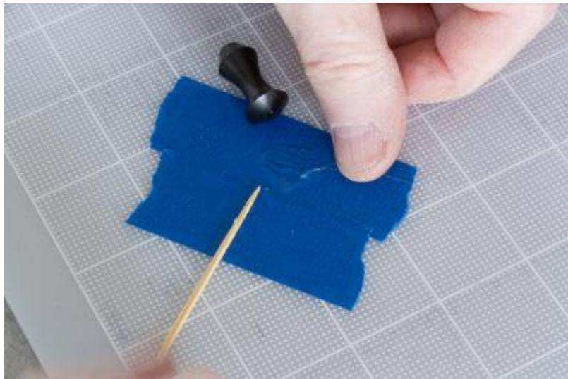
I use epoxy for all of my fastening needs on ornaments. I like the open time, the ability to fill gaps, and the long-term flexibility of the material. The hole has been wetted with glue and here the knot is coated with glue as well.
