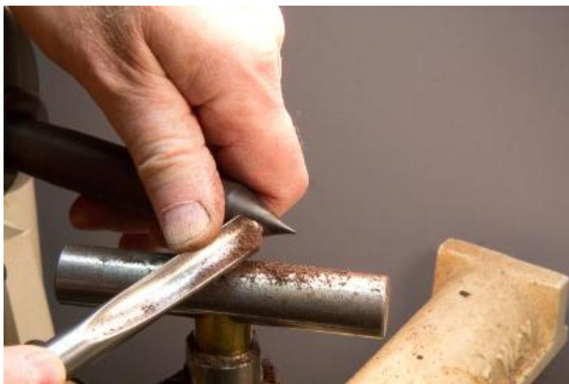
A more effective way to cut delicate spindles, mounted only from one end or between centers, is to support the cut with your own "spindle steady". If you "squeeze" the work between the cutting edge and your spindle steady, there is no reason for it to flex. It only rotates between the two equal and opposing forces.
