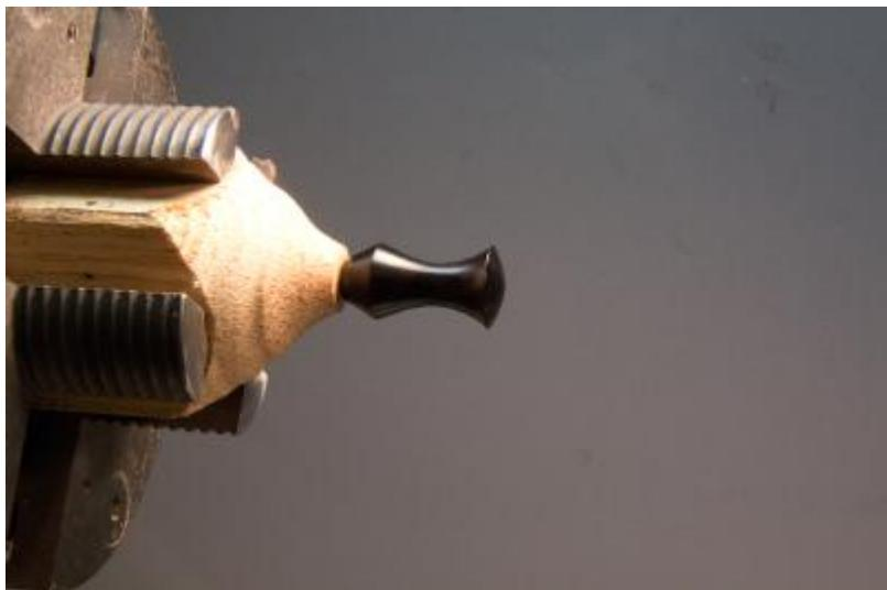
Turned, sanded, and finished. When running on a stub of a mandrel like this, sharp tools and light touch are the keys. These are good skills to develop regardless of your turning interests. At this point, time for a quick center drill and then drilling for hanging line.
