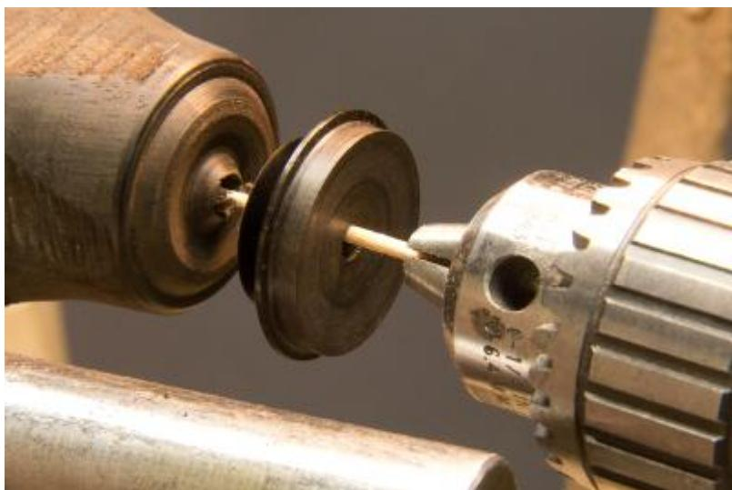
Top and bottom finial "bases" are turned as much as possible when mounted in the chuck. Then are parted off and reverse mounted in the chuck for completion on that side. The small inner diameter on each can be marred in work holding as they are internal. Here a toothpick is used to capture the bottom plug on separation.
