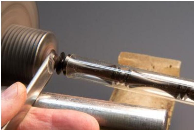
With your “catchers mitt” in place, you can now focus on finishing up the details at the interface end of the finial. You can also support your tool properly having both hands available to control the tool and make the separation.
