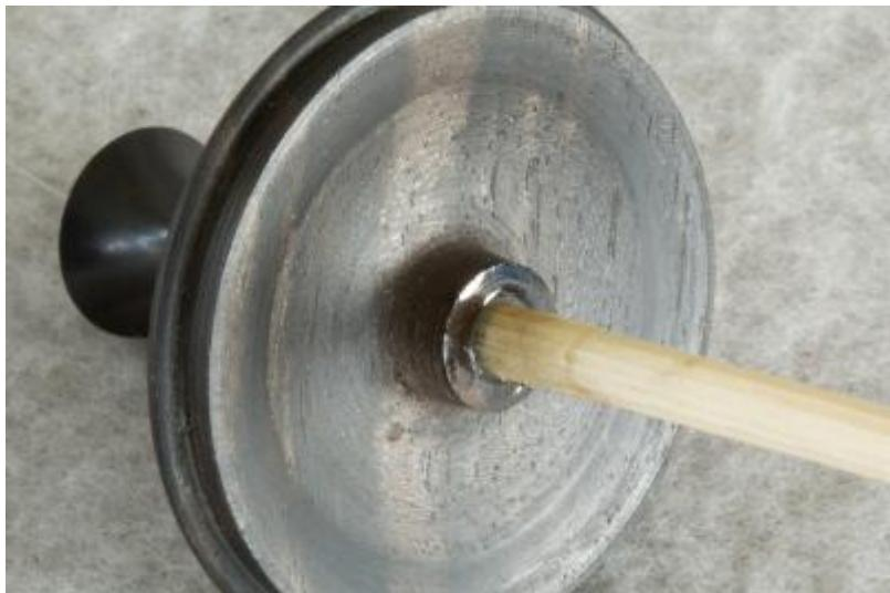
Once the top finial is cured, it is time to add the top finial base. Because the interface between the top finial and the top finial base is a visual interface, all adhesive is applied on the inside bottom. There is no load on this joint so it only needs to be held in place.
