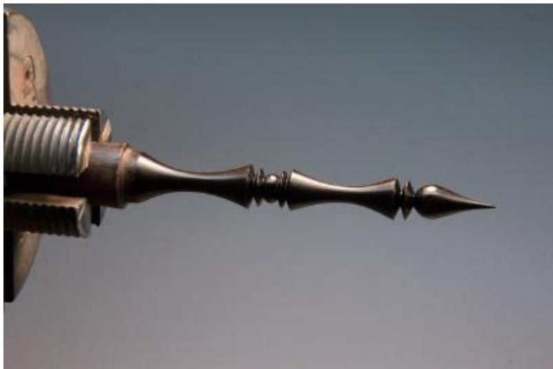
Ready for parting off. Remember, prior to this mounting, the blank was rounded to run true, mounted, faced, and the kabob hole was drilled to a planned depth. I already know where the end of the finial must be to be properly assembled.
