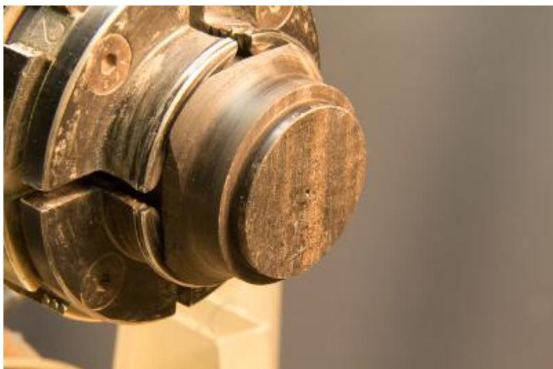
Here is the bottom of the top finial “base”, the piece that will fit into the opening of the shell. There is a shoulder to rest on the top of the shell as well as a bit of an inside “plug” to help block seeing any flaws in that opening of the shell.
