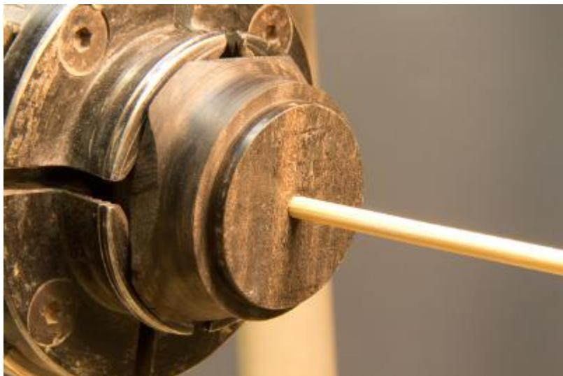
Even though it isn't a critical dimension or fit, it takes little time and effort to test fit the actual kabob skewer that is intended for use. If there isn't sufficient clearance for loose slip fit, drill larger. Too much clearance? Change kabob skewers for one in the bag with a larger diameter.
