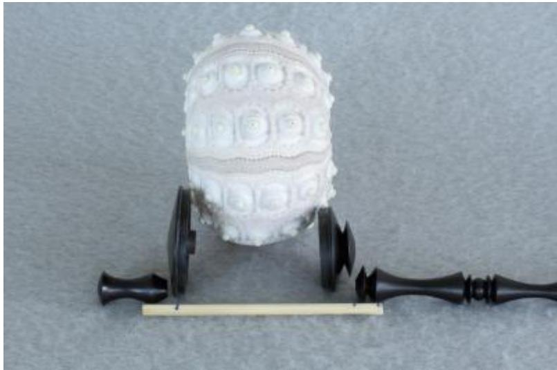
Here are all of the parts of my ornament assembly. Top finial, top finial base, shell (of any kind), bottom finial base, and bottom finial. All of the pieces that will be held together with a piece of bamboo kabob skewer. No wasted wood by turning little finials out of much larger diameter stock.
