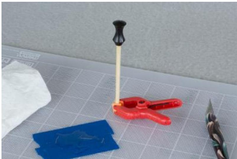
A high tech curing fixture. The weight of the finial keeps it seated while it cures. Also by standing it straight up, there is little tendency for the kabob skewer to not remain centered should the hole be a touch large. The flared out fibers also help keep things centered.
