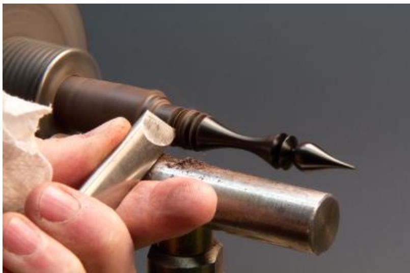
Work in small sections and work to completion while progressing towards the headstock. Also notice the paper towel. No cloth in my shop for safety reasons. The paper towel is used to clean the turning between each progressive grit of sandpaper.
