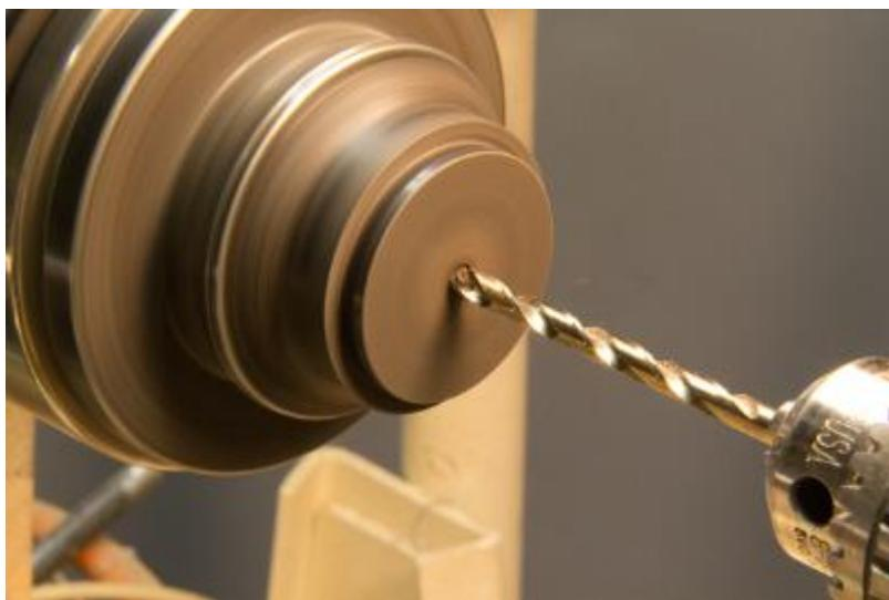
I use a piece of bamboo kabob skewer to hold my many ornament component pieces together. Here is the drilling to pass the kabob skewer through. The diameter is drilled to be a slip fit to allow for gluing.
