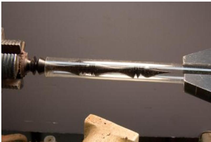
A more appropriate sized “catchers mitt” and a smaller chuck to hold it in place. There is no contact between the finial and clear tube so there is no need for the tailstock to rotate. The tube is only there to catch the finial to prevent damage when parted off.
