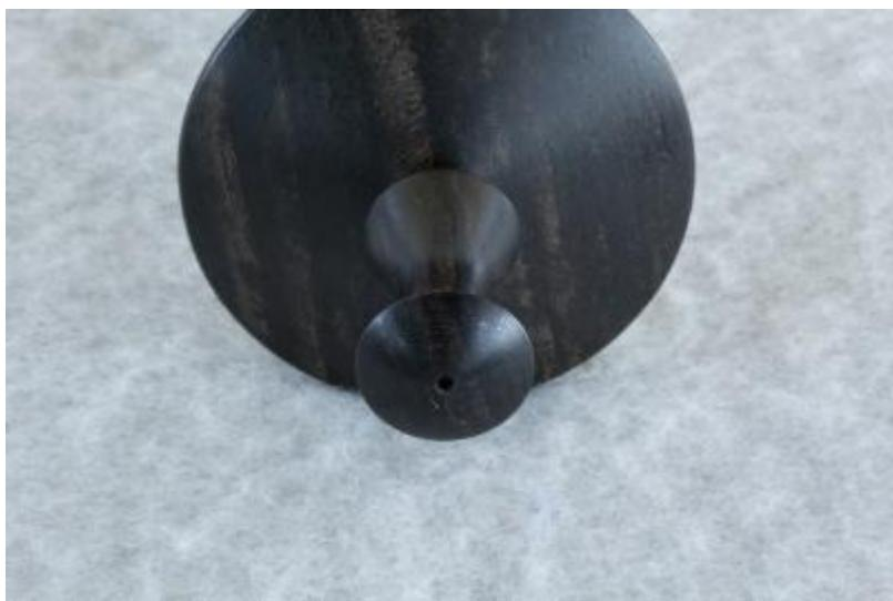
Even though my frugality has made me use two different pieces of wood to create this finial, it never hurts to line up the grain as much as possible while gluing things up. Attention to detail does make a difference.
