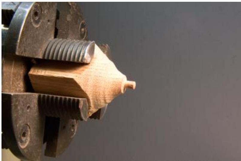
Custom turning mandrels as needed is a worthwhile skill to develop. Here a scrap piece of oak is used to make a mandrel for the finish turning of the upper finial. The finial was already drilled for the kabob diameter and that hole is used for the mounting on the mandrel.
