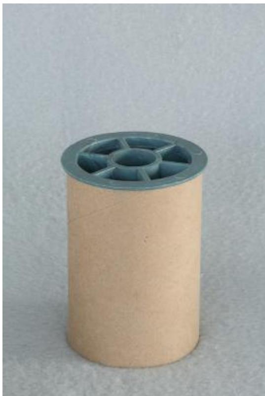
Another high tech assembly fixture. A cardboard core from a copier paper roll. I cut them down and use them for ornament shipping containers. Here is a short cutoff length with the spindle core in place. The shaft hole becomes a perfect positioning device for positioning the ornament for gluing and to let it rest until cured.
