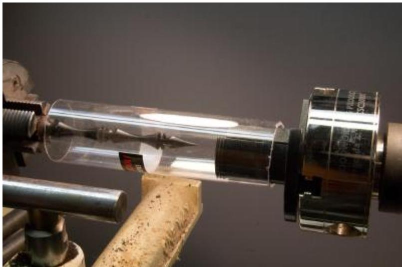
Putting a protective shield around the turning allows for parting off without worrying about reaching over the lathe or having it damaged by falling. This tube, far too big, is better than nothing.
