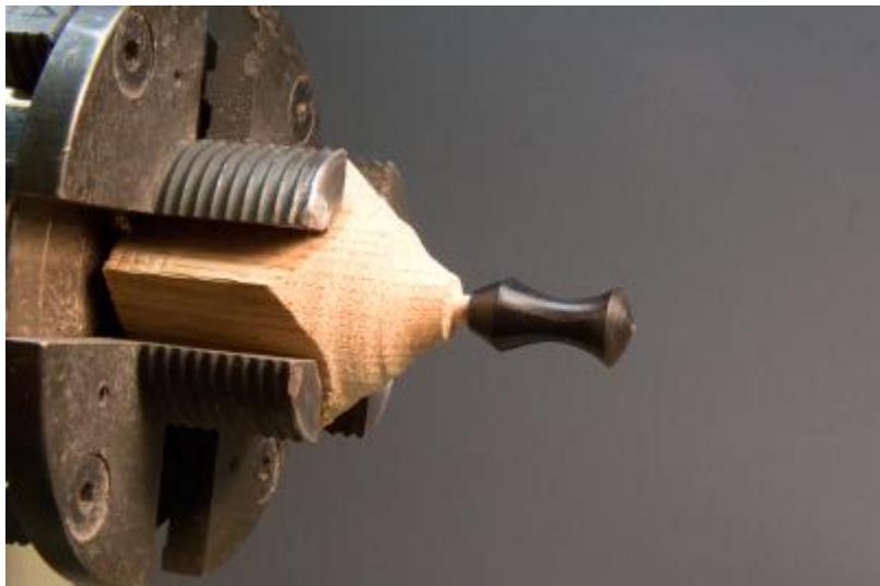
Unless the walls of your finial are thin or weak, you can cut the mandrel shaft size to be snug press fit. If you are too loose, re-cut another piece or wet the mandrel before putting on the finial.
