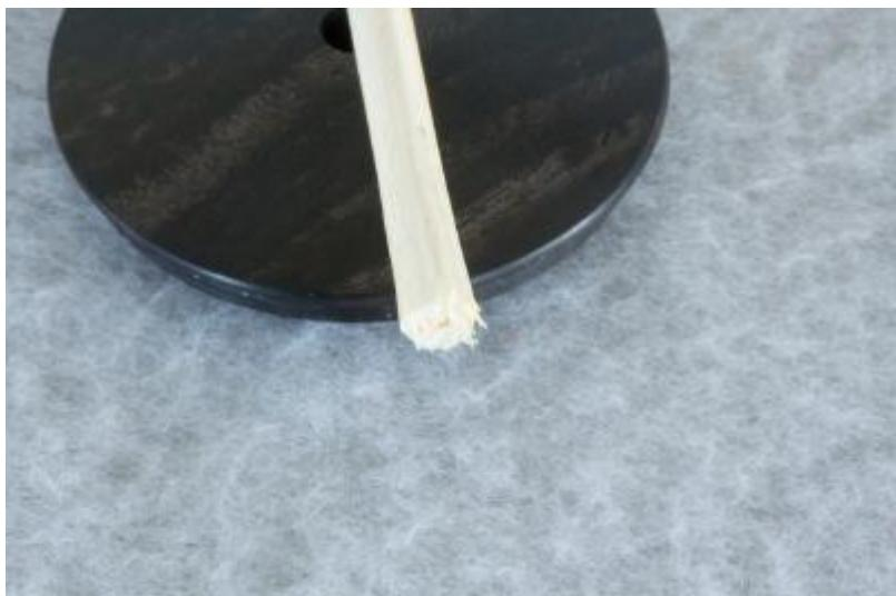
Bamboo kabob skewers are nearly impossible to cut cleanly so I use this to my advantage. The raggedness can help gap fill as well as provide more face grain surface for adhesion.
