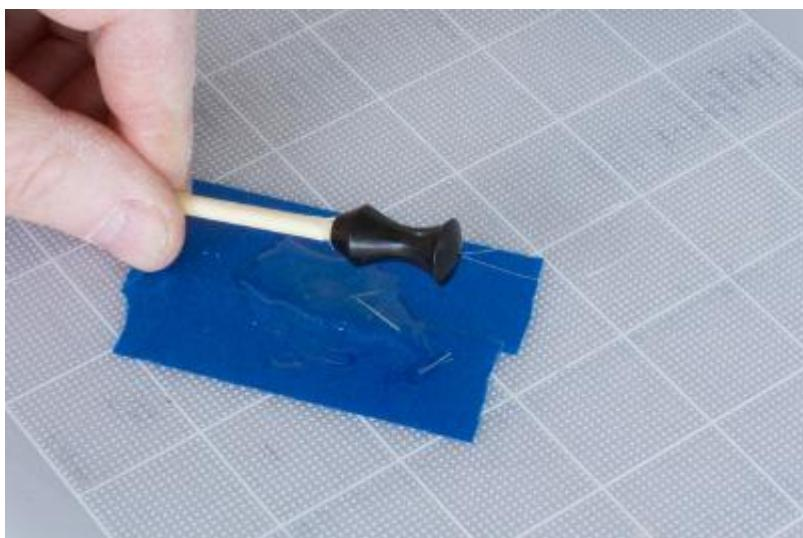
The kabob skewer is bottomed out in the top finial, twisted around to spread the glue, and set aside to cure. Care is taken to keep the area on the bottom surface of the finial clean. This will be a mating surface to the upper finial base. Good clean mating surfaces will help the visual appearance.
