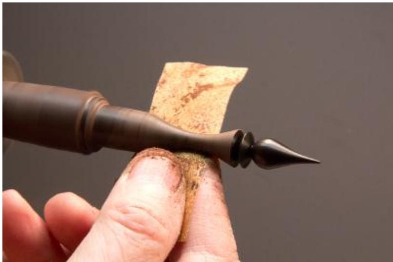
Work from the tailstock end towards the headstock, turning, sanding, and finishing in small sections as you go. Leave as much strength as you can for as long as you can. This is a one-way trip. Get everything just the way you want it before moving on to the next section.
