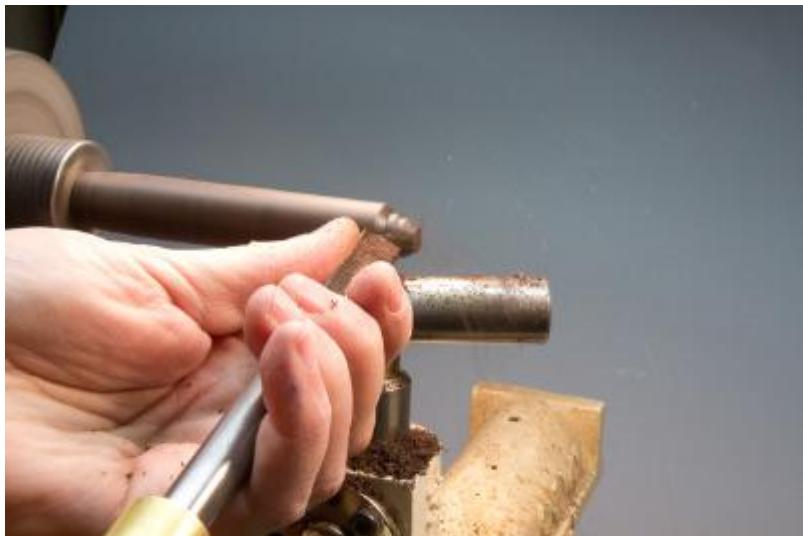
For my bottom finial, I always turn with only a headstock mount. No tailstock. That allows it to run true and have no incentive to flex because of tailstock compressive forces. Traditional spindle cutting with that much unsupported length usually doesn't work very well.
