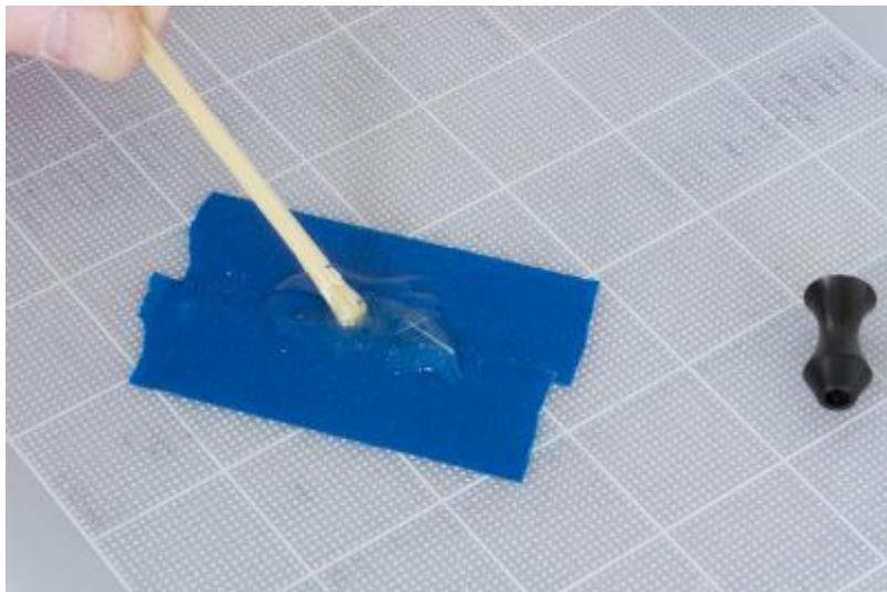
With the ends crushed, why not use the kabob skewer as my mixing stick? Saves getting something else dirty and helps work the adhesive into all of the fibers on the crushed end of the skewer.
