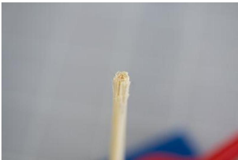
I intentionally crush both ends for the reasons above. Originally, I used the parent finial material turned to a tenon and glued into the top. That developed into assembly with a dowel, and then a thinner dowel to now kabob skewers. The kabob skewers, or something similar, are cheaper, smaller, and lighter. Certainly strong enough for those turning beastly ornaments but works well in all sizes of work.
