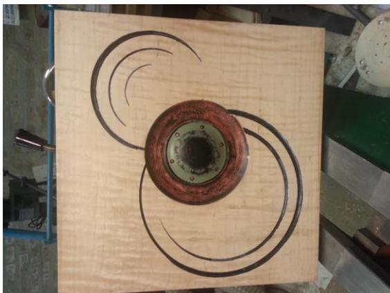
Remove the plaque from the lathe and lay it on a padded surface. Unscrew the faceplate. Remove the sacrificial mounting wood by tapping a wide wood chisel around the outside. Tap the chisel in the direction of the long grain so that the finished plaque won't split. Once the plaque is removed inspect the back side and decide if the back should be sanded or not.
