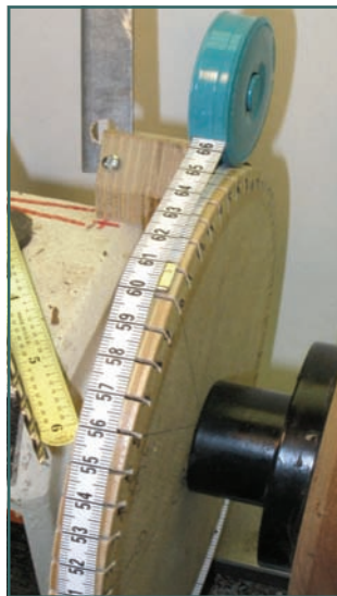
Laying out 60 divisions
