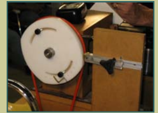
The MDF Lathe showing the rosette (cam) and rubber (cam follower)
