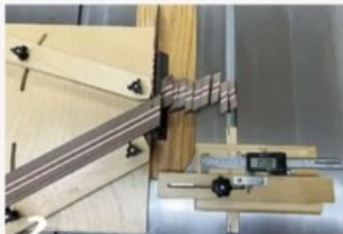
The author uses a Wedgie Sled (shown at left) to cut a lamination at a 30-degree angle. At right is a stop, which ensures all of the pieces are of identical size.
