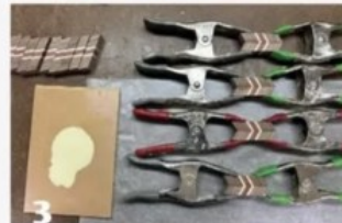
Glue the cut pairs into a single zigzag, also called a chevron.
